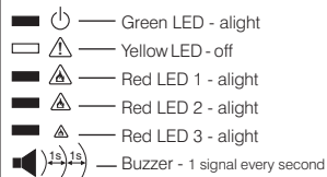
Fig. 6 - "Gas presence alarm" status
